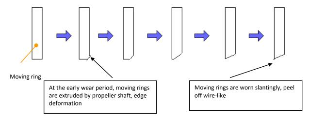
① The mechanical structure of the machine, sometimes may cause stripping of "burr" on the moving ring, The degree shown in the photograph below has no effect on the structure and performance of the machine.
