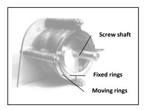
The gaps between the fixed rings and moving rings, and the pitch of the screw narrows down gradually from the concentration zone to dewatering zone, The thickened sludge was transferred to the dewatering zone, in this zone, the gaps between the rings and screw pitch gradually narrow, and the end plate blocks the flow, thereby, narrowing the volume and increasing the pressure encourage the dewatering process.
