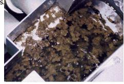
(7) Flocs flows into the screw press and discharged from the outlet as sludge cake
