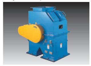
A rotating drum eliminates magnetic foreign bodies from particulate raw materials and products.
