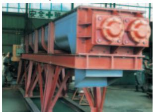
This conveyor uses a rotating screw to move the load.
