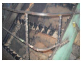
**Intermediate Carrier** P=304.8mm Intermediate carrier chain
