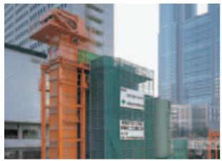
A bucket elevator designed with the properties of mud in mind, with a simple structure for easy maintenance and repair.
