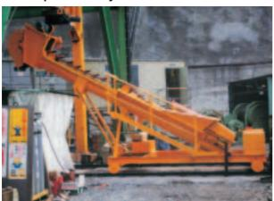
A conveyor ideally suited for ready-mix concrete and sludge.
